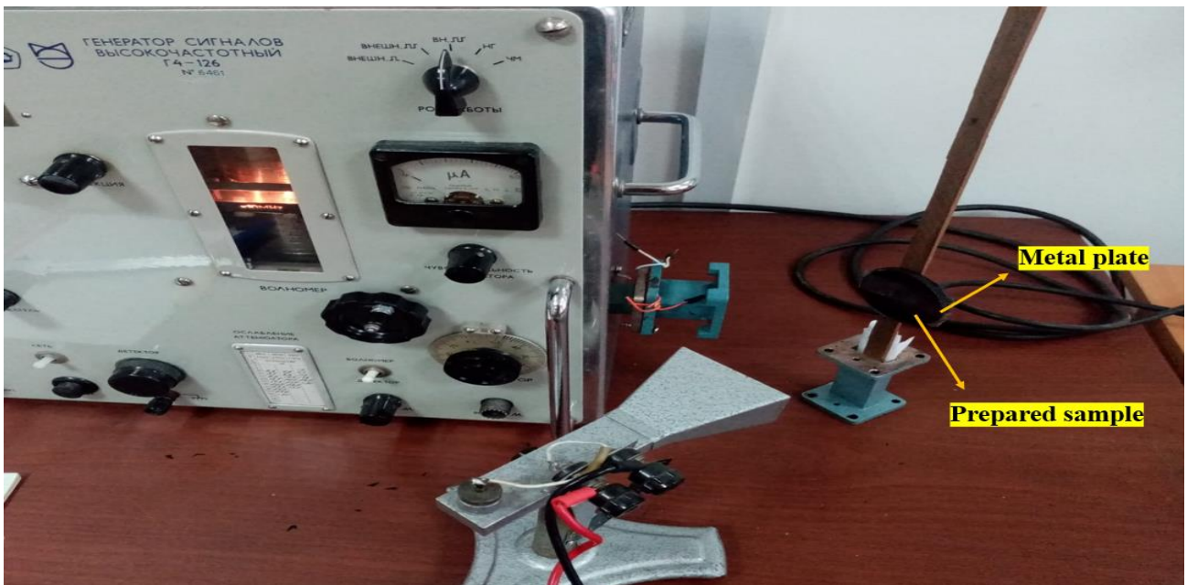
Figure 10 – Experimental setup for measuring the reflected power of the EM waves for the microwave absorption model
